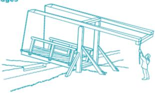
Pull the chain hanging from the balance arm. When the bridge is open, unless it's obvious that there's a mechanism to stop the bridge from lowering by itself, sit an adult on the arm to keep it raised until the boat's clear of the bridge.
