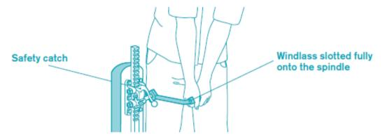
With one crew member at the helm and one at the paddles, you wind the paddle gear up and down using a windlass or lock key. You should always wind them bit-by-bit – and keep an eye on the effect of the moving water on your boat.
